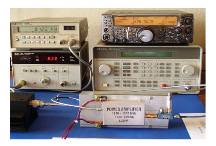
Amplifier prototype, compression test
