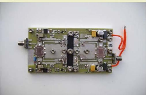
Amplifier mount on the heat spreader, pallet size 90 x 56 X 16 mm
